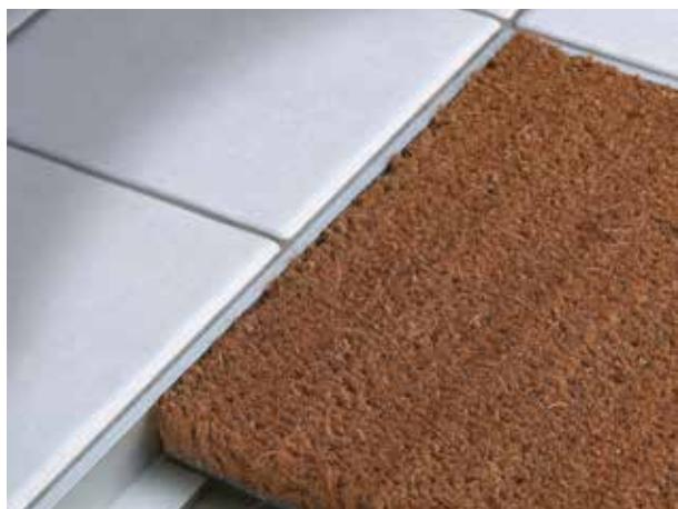
Reversible profile to create perimeters suitable for containing doormats. The profile accommodates the two most common doormat thicknesses of 18 and 23 mm. Installing the frame must be done at the appropriate height before the installation of the adjacent flooring material. The profile can also be installed using modular and sliding fixing brackets inside the slots.
